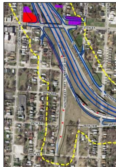
Proposed Split Diamond Interchange between 27 th Street and Jackson Curve (See Figure 2-1)
