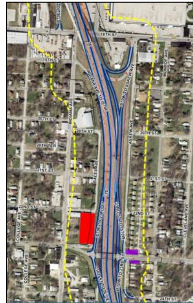
Proposed Separated Auxiliary Lane between 18 th Street and 23 rd Street (See Figure 2-1)
