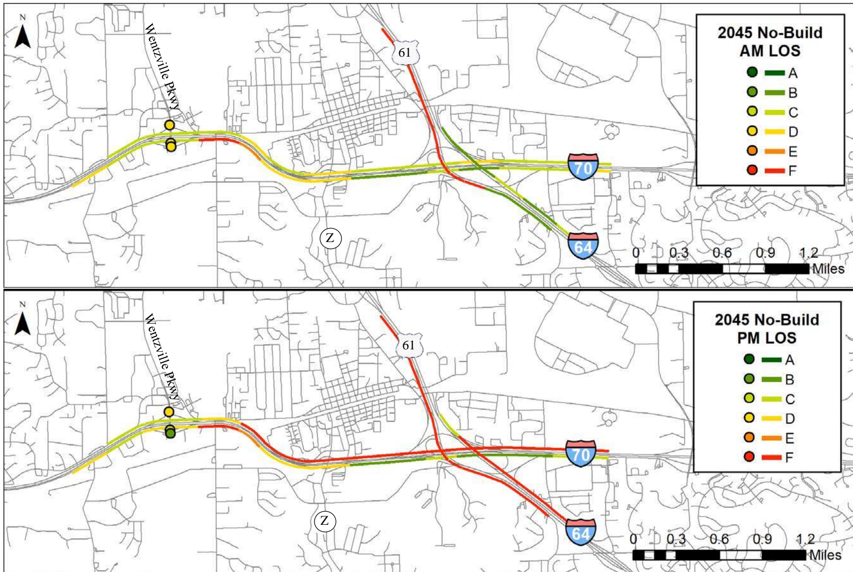
Figure 20: 2045 No-Build Freeway LOS Conditions for AM and PM peak hours
