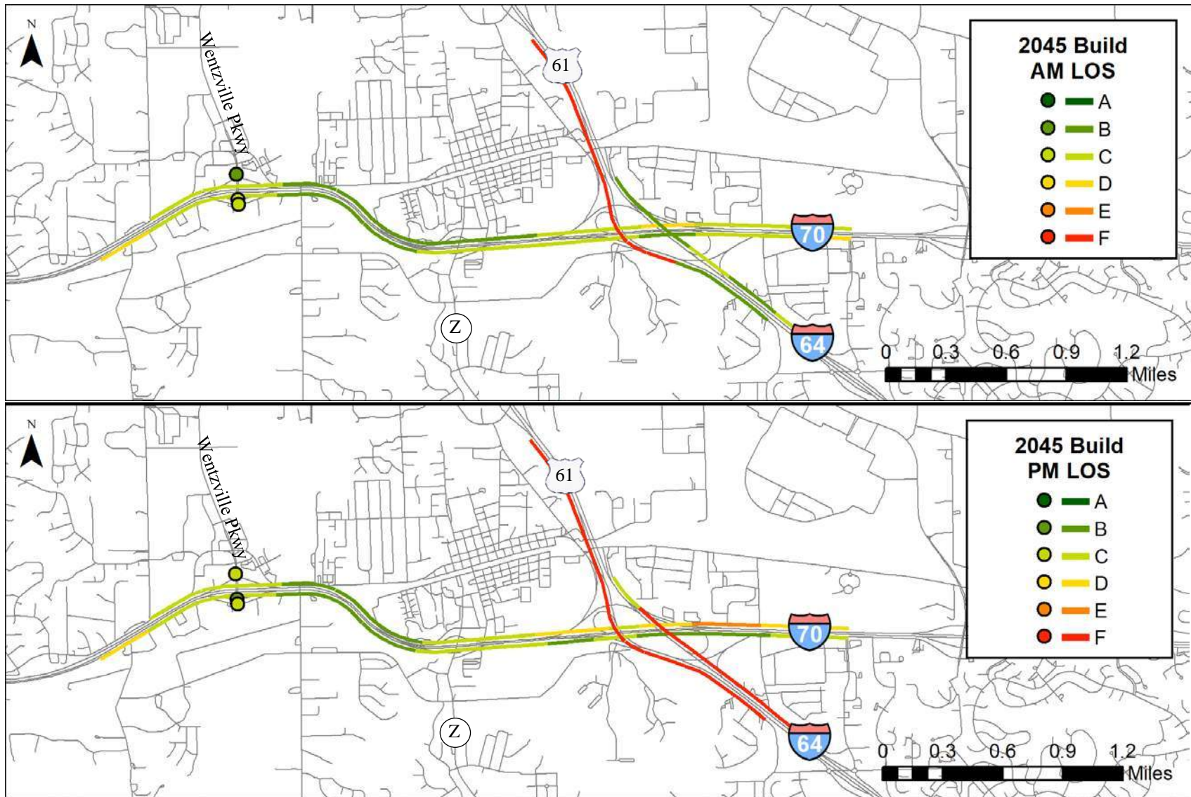
Figure 21: 2045 Build Freeway LOS Conditions for AM and PM peak hours
