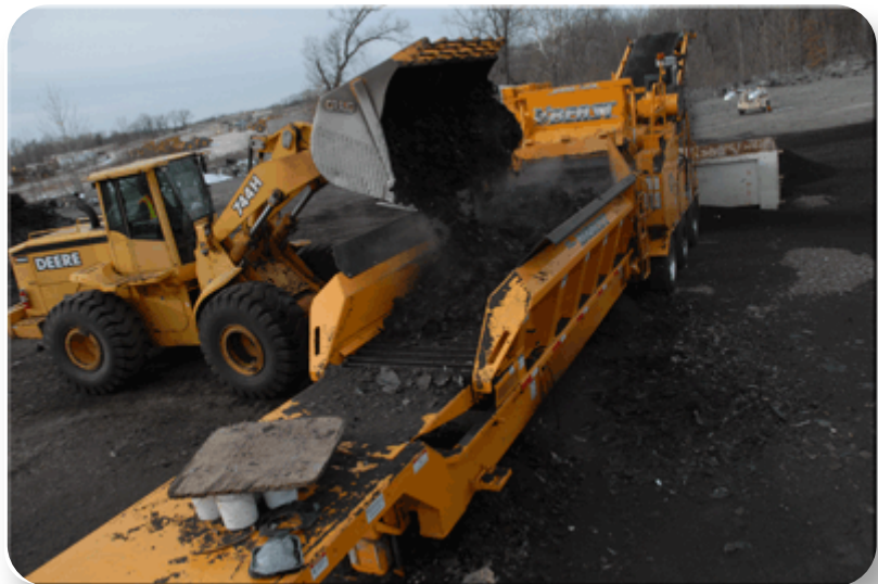
Shingles are ground up and processed
