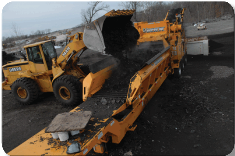
Shingles are ground up and processed
